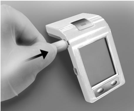
1. Insert the probe cord completely into the jack on the left side of the Root ZX mini.
