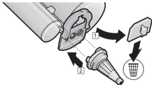
2. Remove the cap from the cartridge and discard. Attach a new mixing tip.
