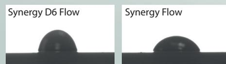
To compare the flow properties, 5mg of Synergy D6 Flow and Synergy Flow were extruded and photographed after 20 s.
